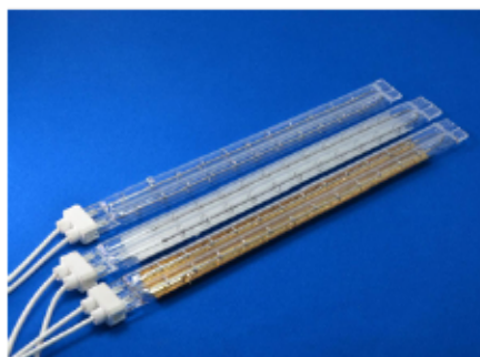
Twin Tube Short Wave IR Quartz Lamp Voltios: 110V ~ 600V / Watts: 500W ~ 16KW Twin tube: 23×11mm, 33×15mm Reflector: Ceramic white or Gold Densidad máxima de potencia: 200 kw / m 2
